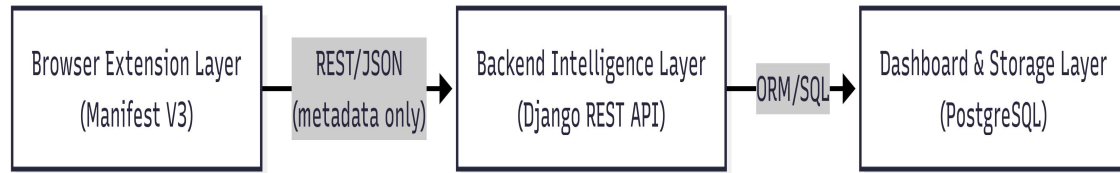
Fig. 1. Three-tier architecture: the Browser Extension Layer communicates with the Backend Intelligence Layer over a metadata-only REST/JSON API, which persists results to the Dashboard and Storage Layer via ORM/SQL.
